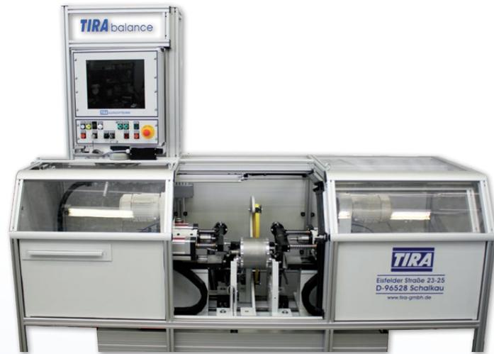
Balancing technology is necessary, when mass unbalance of rotating parts or tools have to be removed or minimized.
