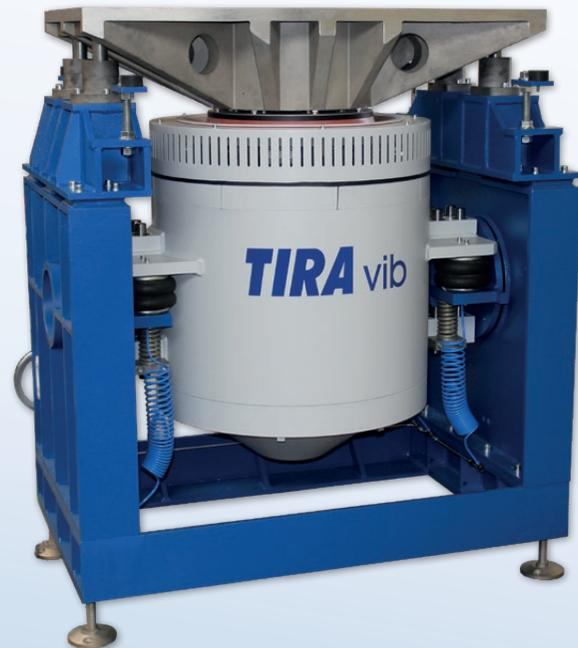
Vibration test systems from TIRA are developed for implementation of generally accepted standards MIL, ISO, ASTM, EN and DIN, for application within different industry branches and at the introduction of new technologies.
